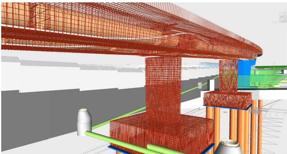
Pilot-project: Viaducts of Campo Grande, in Lisboa (rebar cages 3D modelling)
